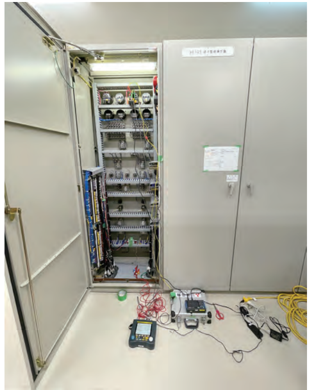
図9 始動電流および力率測定状況 Fig.9 CFD analysis of pump model
