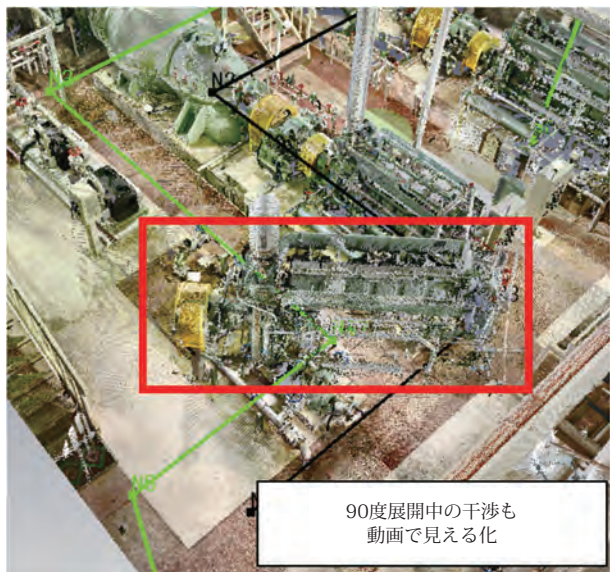
図6-2 干渉確認図 Fig.6-2 Collision simulation
