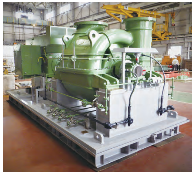
図3 Thermal oxidizer air blower外観 Fig.3 View of thermal oxidizer air blower
