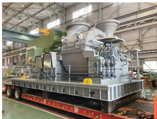
図3 ブロワ外観 Fig.3 View of Combustion air blower
