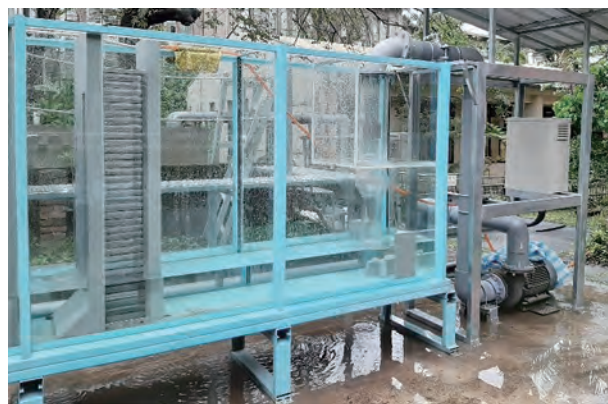
図8 模型水槽 Fig.8 Model Sump
