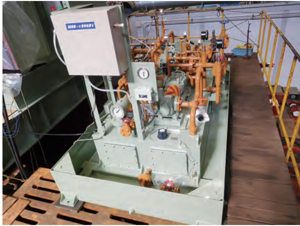
図6 強制給油装置外観 Fig.6 View of-Lube Oil System
