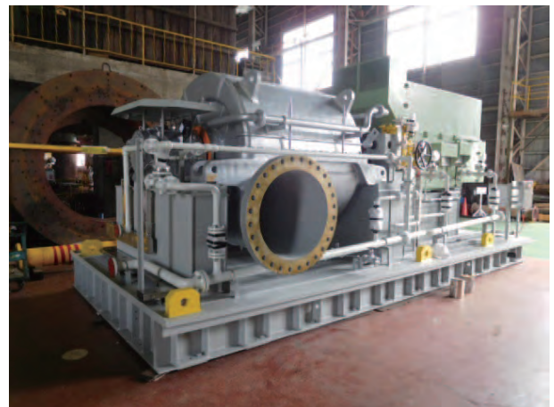
図3 Claus Air Blower 外観 Fig.3 View of Claus Air Blower
