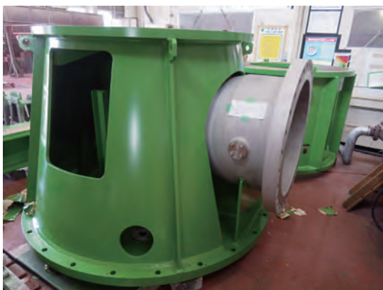
図5 吐出しエルボ外観 Fig.5 View of discharge elbow
