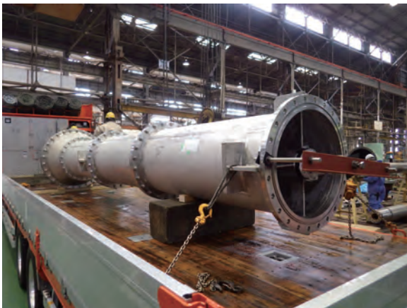
図4 温水ポンプ横外観 Fig.4 Sidewise view of Hotwell pump
