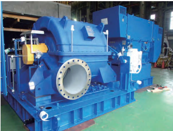
図2 Main Air Blower 外観 Fig.2 View of Main Air Blower
