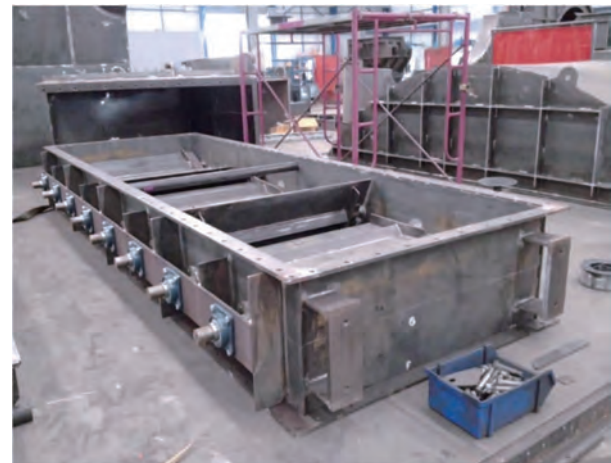
図4 吸込ダンパの製作状況 Fig.4 Manufacturing for suction damper
