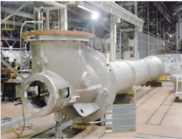
図2 気化器海水ポンプ外観 Fig.2 View of sea water vaporizer pump
