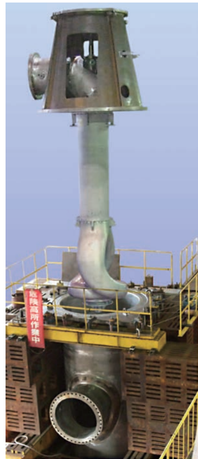
図3 Hotwell pump 外観 Fig.3 View of Hotwell pump
