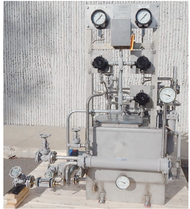
図3 強制給油装置外観 Fig.3 View of lube oil unit
