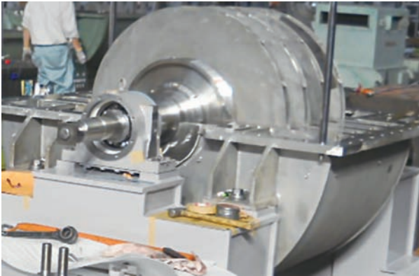
図2 上ケーシング分解状態 Fig.2 View of dismantled condition
