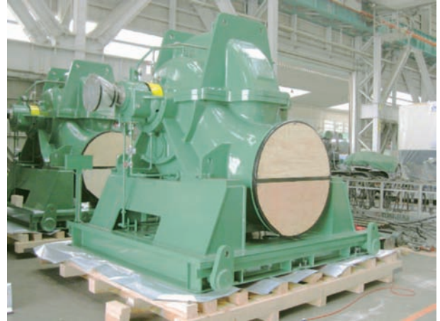
図18 Cooling water pump
