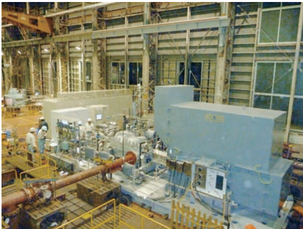
図2 ポンプ工場試験状況外観 Fig.2 Outline view of Mainline Pump during FAT
