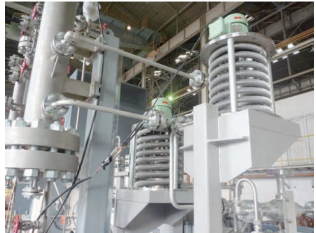
図5 バッファ液用空冷式冷却装置 Fig.5 Air cooling system for buffer liquid of Plan 52
