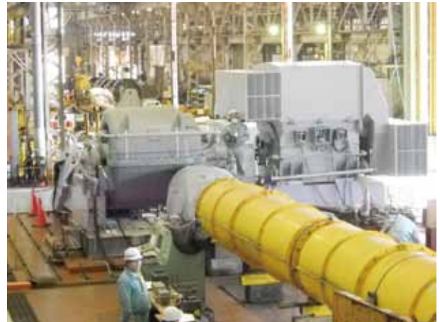
図9 ブロワ性能試験 Fig.9 View of Performance Test for blower
