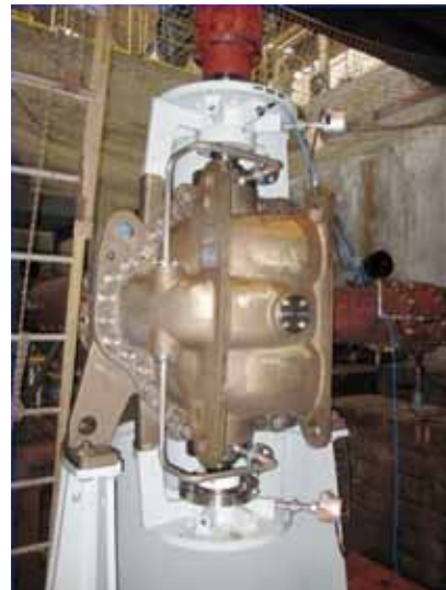
図4 社内試運転 Fig.4 Shop performance test
