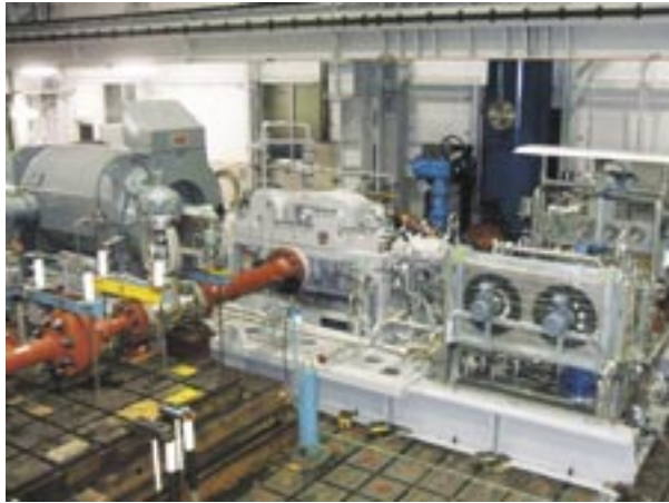
図2 ポンプ工場試験状況概観 Fig. 2 Outline view of main oil line pump at shop test
