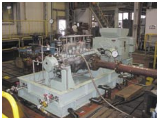
図4 社内試運転 Fig. 4 Shop performance test
