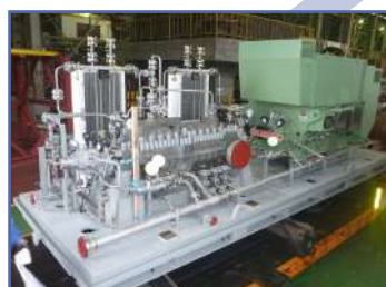
Water Injection Pump
