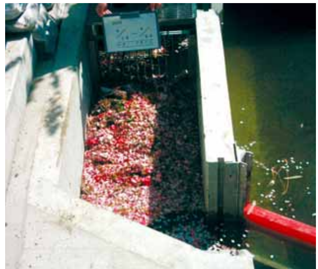
図11 浮遊ゴミの集積効果確認状況 Fig.11 Effective confirmation of accumulating float rubbish
