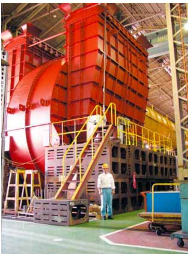
図2 誘引通風機外観 Fig. 2 View of IDF
